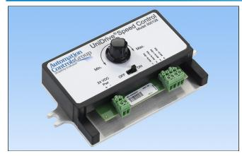
The 300128 Speed Control provides an adjustable 1VDC - 9VDC analog output for use in controlling the speed of up to ten 110515 or 110546 UniDrive<sup>®</sup> motor controls using only one 300128 Speed Control. The 110515 and 110546 motor controls require a differential analog input signal and the + and – analog output from the 300128 Speed Control provide this differential signal.
